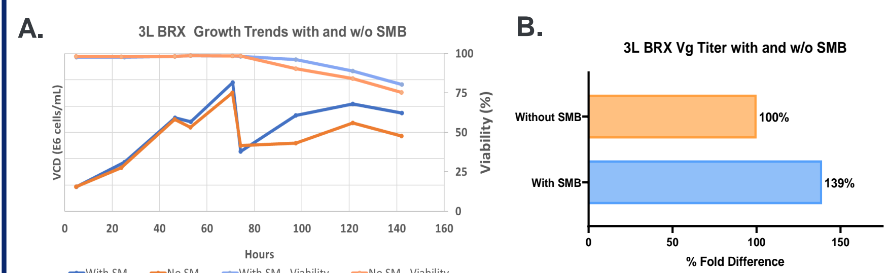
Figure 4. 3L BRX Results with and without SMB A. Viable cell density and % viable cell density was comparable with and without SMB B. Vg titer with SMB increased by 39% compared to without SMB in 3L BRX C. Metabolites were comparable with and without SMB in the shake flask satellites.
